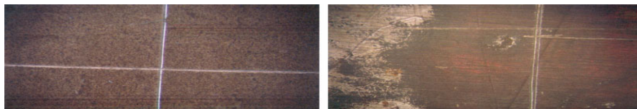
Figure 10 Microscope images of PBIs coated on metal surfaces after the adhesion test: PBI-4 (left) and PBI-1 (right). [Color figure can be viewed in the online issue, which is available at www.interscience.wiley.com .]
